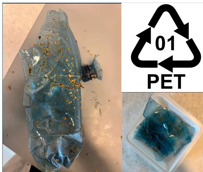
Fig. 6 The photo of plastic (blue PET) litter caught from the Motława river, rinsed with water and dried
