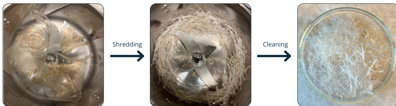
Fig. 5 The images of the sample after shredding and cleaning
