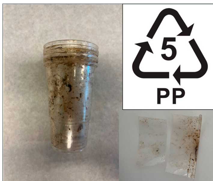
Fig. 1 A photo of plastic (PP) litter retrieved from the Aarhus River, showing the items after being rinsed with water and air-dried.
